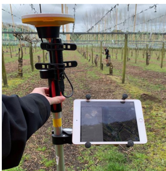
GNSS (Global Navigation Satellite System) RTK (Real Time Kinematic) equipment.
